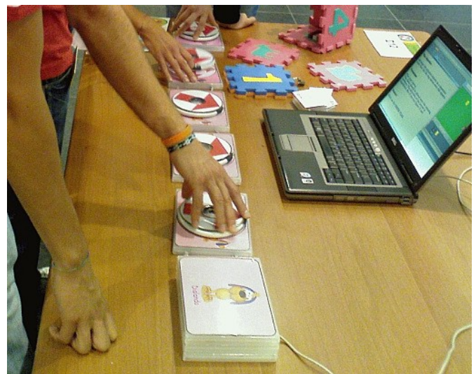
Fig. 7. Dialando is a physical programming system using five rotational inputs to control an on-screen avatar.
