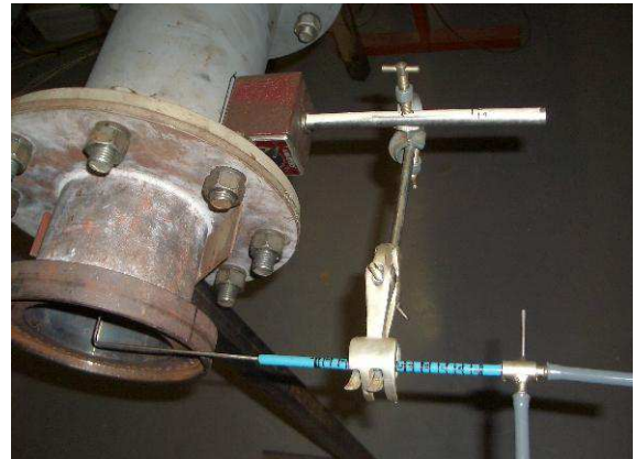
Figure 5: A magnetic clamp holds the Pitot tube onto the test rig in the correct position.
