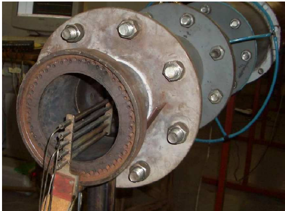
Figure 4: The five K-type thermocouples in a rake at the combustor outlet.
