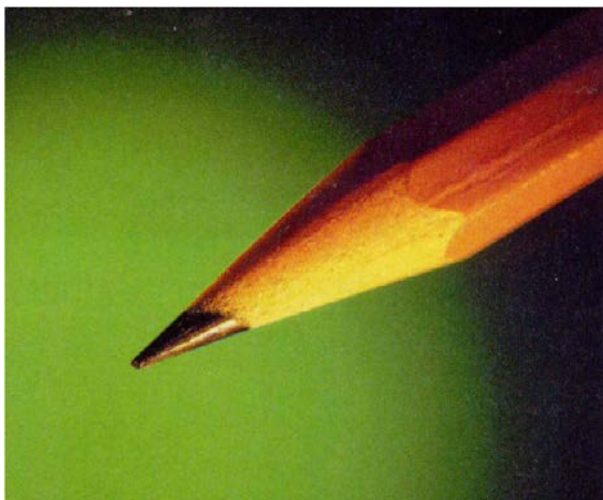
Fig. 9. Graphite in a pencil. When writing in pencil you are placing layers of graphene on paper substrate. Invisible writings could be few layers or even monolayer of graphene. (From A.C. Ferrari et al [7])
