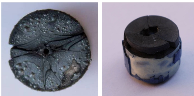
Figure 9: Diamond tools damaged due to the laser heating with both physical and chemical changes evident.
