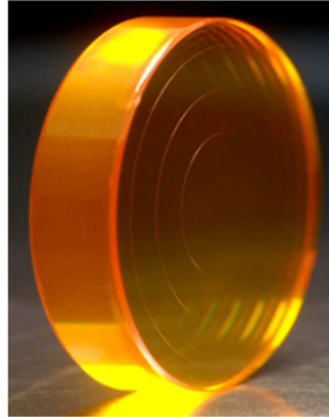
Figure 3: A photograph of the diffractive optical element that was used in this study.
