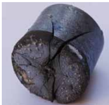
After irradiating with a high power laser beam, an industrial diamond sample is severely damaged by the thermal gradients induced in the sample, with both physical and chemical changes evident.
