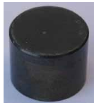
The starting industrial diamond sample is pristine, with a diamond layer on top of a cylindrical base.
