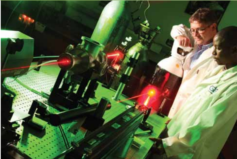
Professor Forbes and MSc student Lerato Shikwambana, aligning the CO 2 laser for laser-material interaction studies.
