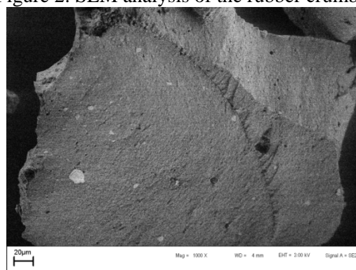
Figure 4: SEM analysis of the rubber crumbs showing surface texture.
