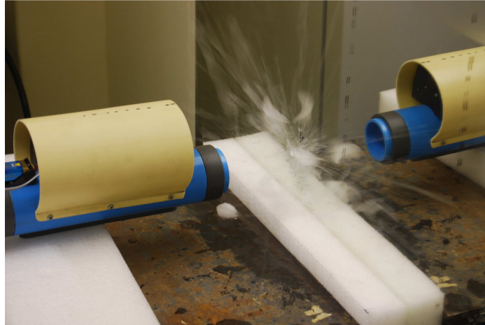
Figure 7: Impact of 45 mm hail stone at 78 m/s
