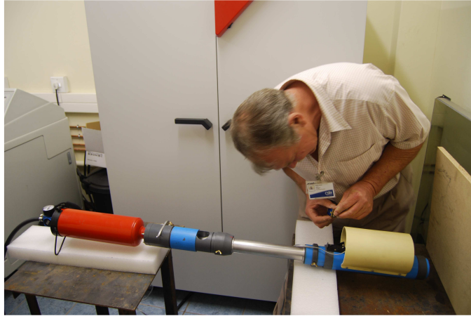
Figure 6: Pneumatic hail gun
