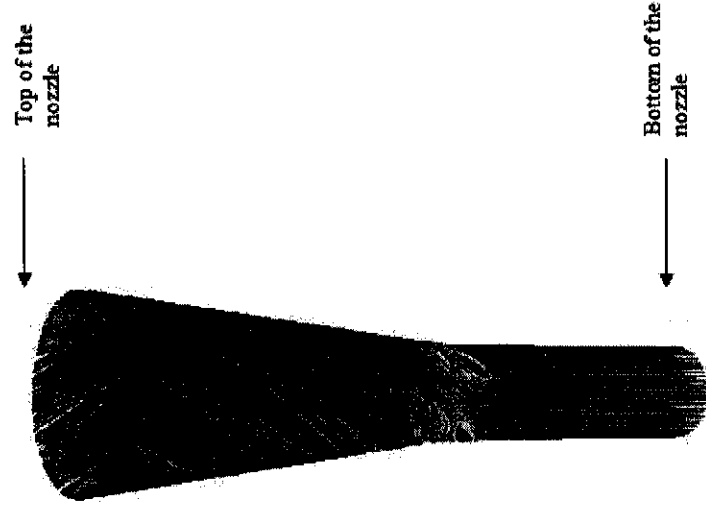
Figure 5. Typical path lines of air inside the nozzle [Source: reference 25]
