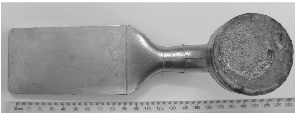
Figure 2. The actual semi-solid rheocast Al-Si binary eutectic plate, including the runner and biscuit
