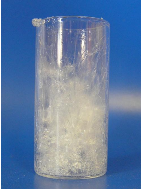
Figure 10: Physical appearance of 30wt% ibuprofen-loaded PEG-PVP complex processed at 60°C
