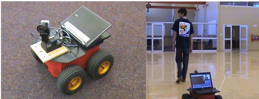
Figure 3.35: The mobile platform on which the work described in this thesis was implemented, together with a still image captured during a following task.
