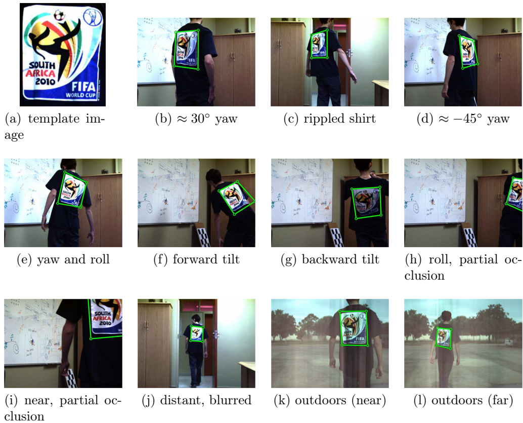
Figure 4.4: Results of the single-view homography-based pose measurement system on a range of test cases. The template image is shown in (a). The superimposed green quadrilaterals in (b)–(l) show the estimated planar approximations from which position and orientation, relative to the template, are extracted.
