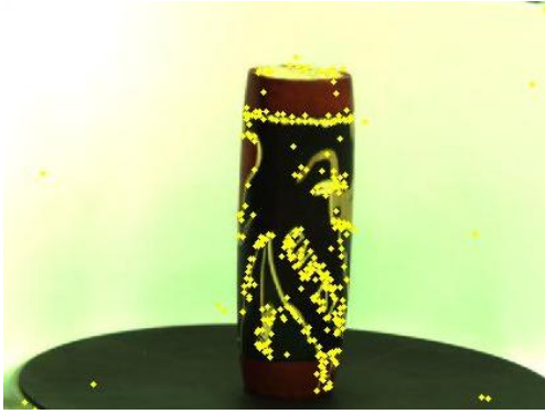
Fig. 1. SIFT features detected and extracted from an object used in the training set
