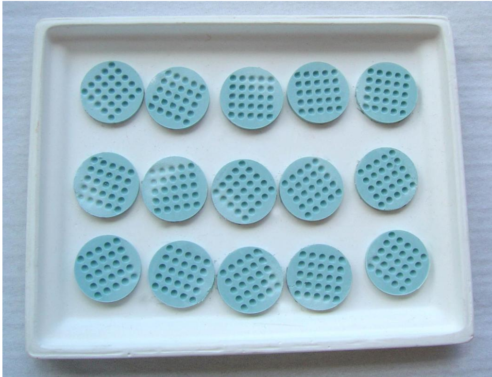
Figure 3: Dimpled HA disks before sintering.
