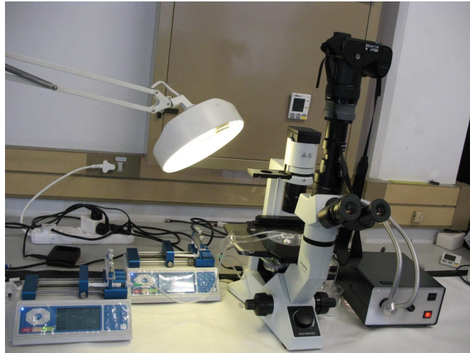
Figure 1: Image of the experimental setup showing two syringe pumps and the microscope.
