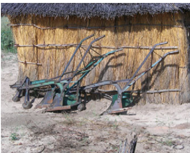
Photo 13: Steel ploughs for ox drawn ploughing. Photo: Alexander Gröngroft.
