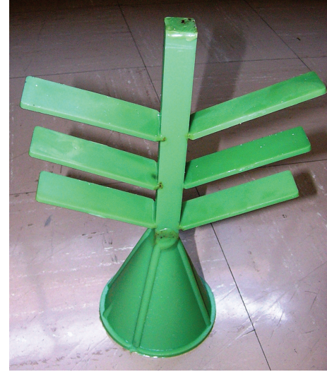
FIGURE 1: Wax pattern assembly used for IC of alloy A356.
