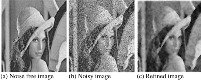
Figure 8: Validating our refinement approach with the popular 2D Lena image [11], (a) Noise free image, (b) Noisy image, and (c) our refined image result.
