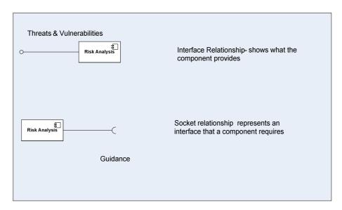
Figure 5: Key to reading Component Diagrams
