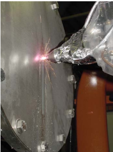
Figure 6: Crack sealing of 4.5 mm plate @ 2 bar pressure.
