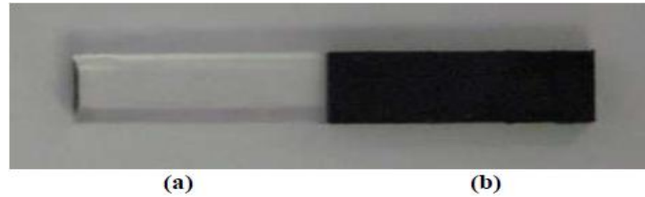
FIGURE 1. Tensile bond test sample (a) pure PDMS and (b) PDMS-CB composite
