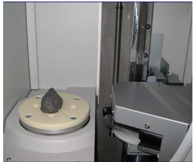
(b) Sample aggregate on rotating table
