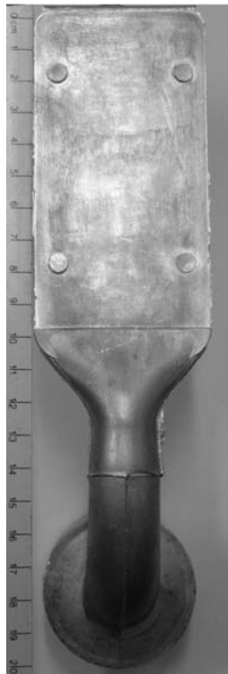
Fig.1 Example of rheocast plate including runner and biscuit
