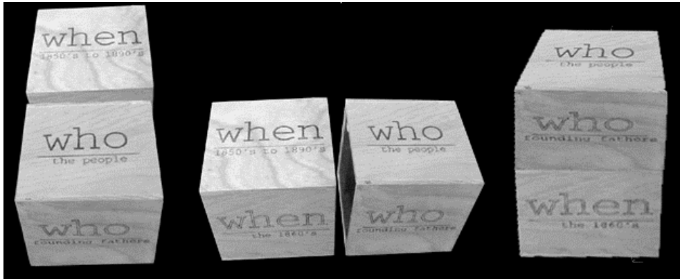
Fig. 20. Using the Navigation Blocks to construct disjunctions and negations. Left: “or” query. Middle: “and” query. Right: “not” query (Camarata 2002)
