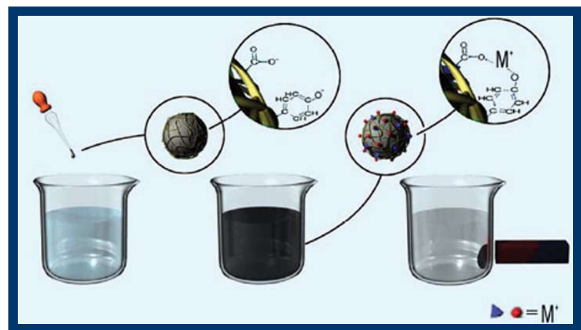
Figure 2: Scheme of removal of heavy metals during water treatment with humic acid coated Fe 3 O 4 magnetic nanoparticles?
