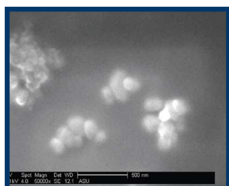
Figure 5: SEM analysis of nTiO 2 in wastewater treatment works (WWTW) tertiary effluent 4
