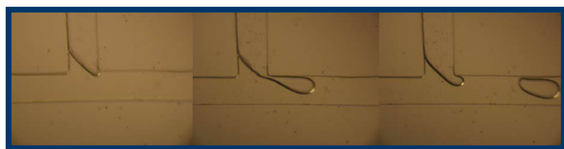
Figure 2: Snapshots showing sequence of w/o droplet breakup in a 200 \mu\text{m} wide microfluidic T-junction
