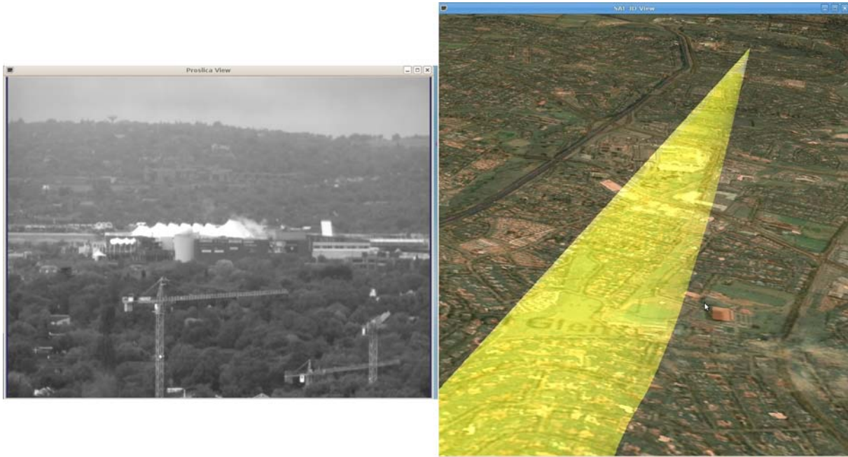
Figure 4: An overview of a live simulation during the development of a pedestal sensor system (DPSS OSS – Image Processing group). The yellow cone is the camera's field of view and the camera image is shown on the left
