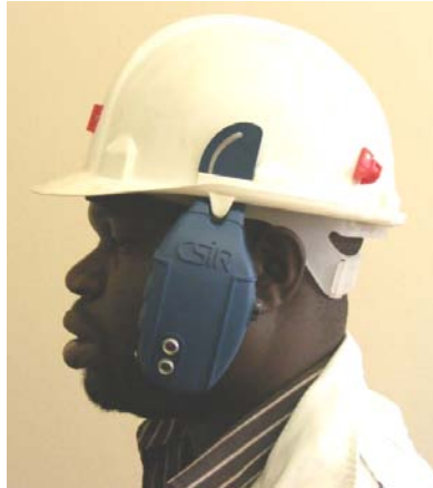
Figure 2. The current manifestation of the Electronic Sounding Device as mounted on a hardhat.
