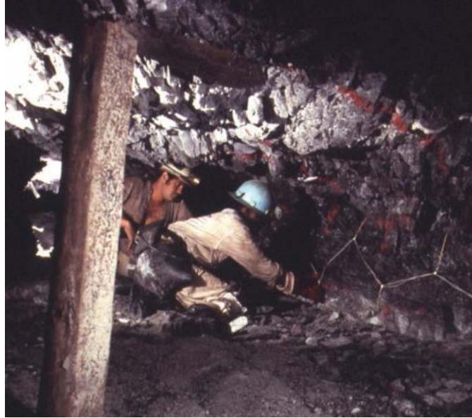
Figure 1. Gold and platinum in South Africa are mined in a thin tabular seam in a hard rock environment.
