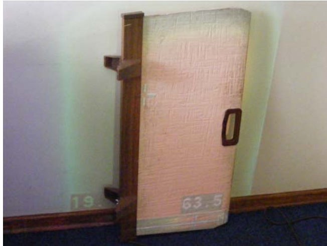
Figure 10. Demonstration of augmented reality: the warm heater is coloured orange by the projector, while the cool wall is coloured blue and green.
