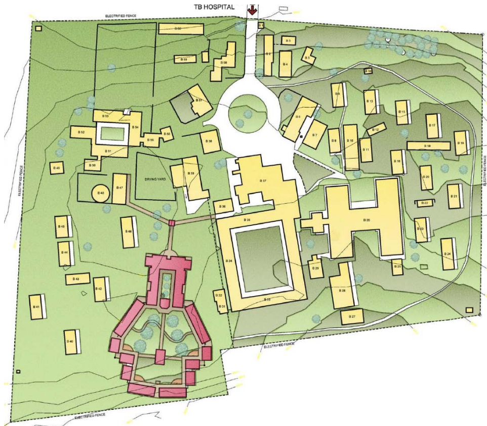
Figure 5: New phase 1 redevelopment at Jose Pearson TB Hospital, Eastern Cape showing existing scattered buildings and the new 40-bed XDR-TB block (red)
