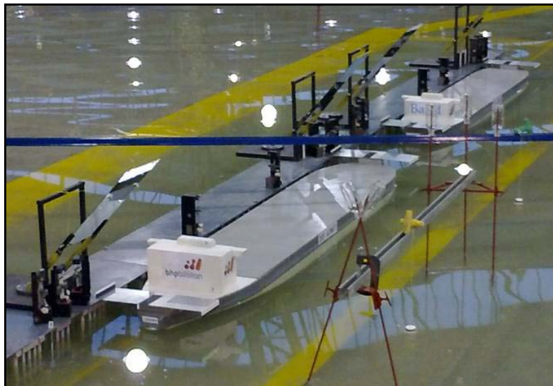
Figure 6: Light metal strips placed on the deck of the model ship
