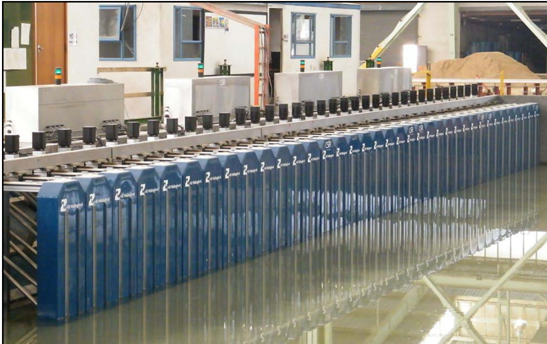
Figure 2: Movable wave generators
