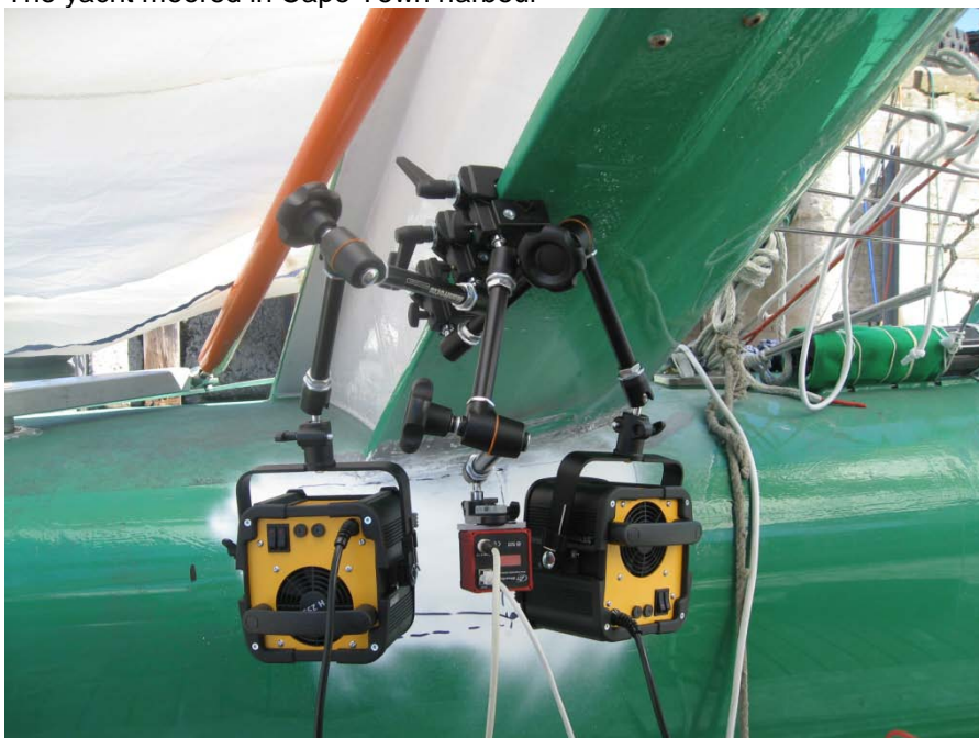
The inspection system affixed to the yacht to eliminate relative motion
