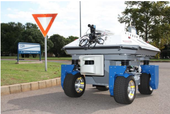
Figure 1: Camera mounted on an autonomous vehicle.
