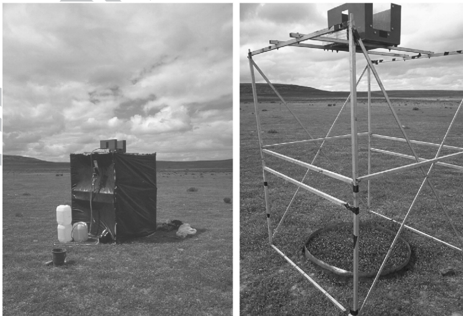
Fig. 5. Single nozzle rainfall simulator used to simulate winter rainfall in September and October 2002 pictured here in managed transformed renosterveld.
