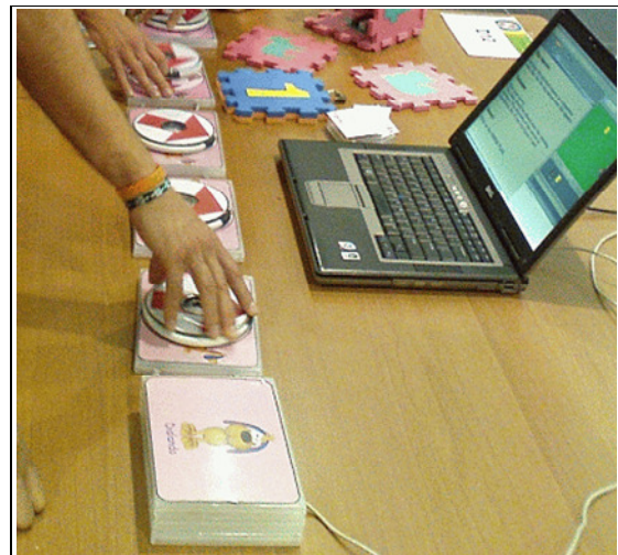
Figure 1. The Dialando programming system in use at a conference demonstration session. The unit at the bottom contains the Arduino controlling circuitry which is connected to the laptop computer using a USB cable.
