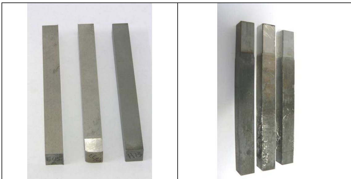
Figure 4: Specimens prior and after 5000 Aluminium Melt Dipping Cycles
