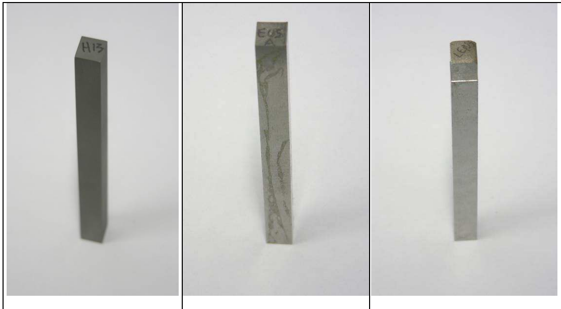
Figure 2: Pictures showing the cores manufactured with the conventional and RP methods From left to right Through hardened steel H13 conventional manufactured specimen, EOS grown specimen, Lens grown specimen
