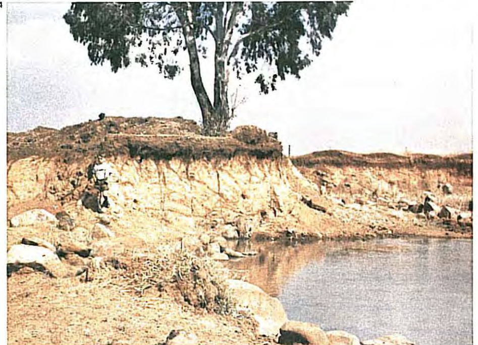
PLATE 14: Highly decomposed dolerite covered by residual black clay. A few dolerite boulders lie on the floor of the pit. Near Dealsville, Orange Free State, where N is about 3.
