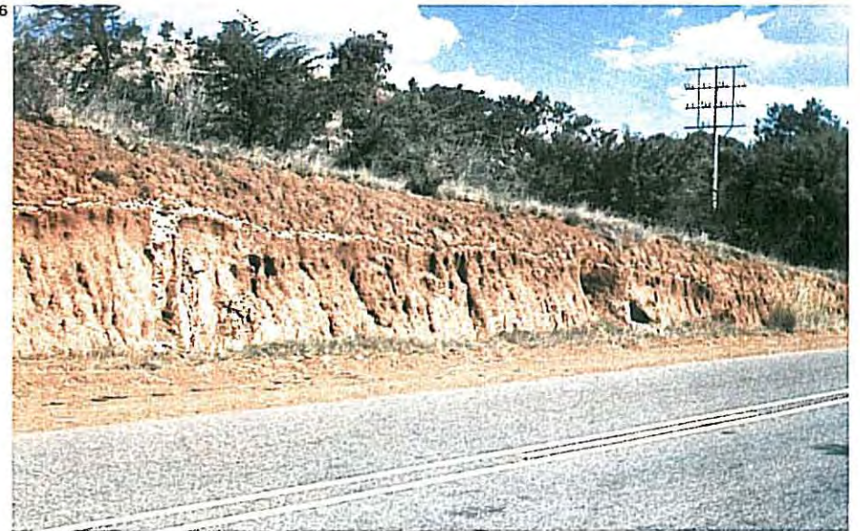
PLATE 6: Pebble marker separating biotic soil above from soil residual from norite below. Note that the quartz veins are cut off at the pebble marker.
