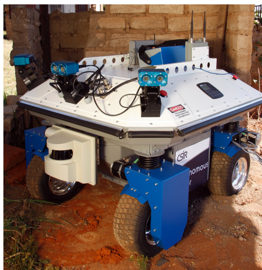
Fig. 1. Seekur, the CSIR Autonomous Rover on which the system was implemented.
