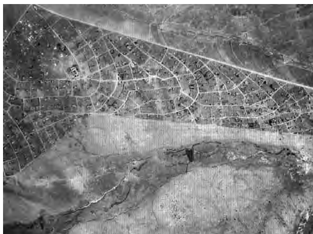
Figure 6.17: The contour-planning concept, to impede the drainage of runoff from the development
