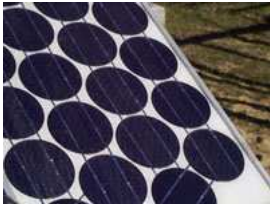
Single-crystalline Si Cell
