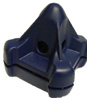
Figure 2. The prototype of an ultrasonic beacon for positioning sensors or mobile sensors underground, together with its housing. The beacon would normally be deployed on the hangingwall.
