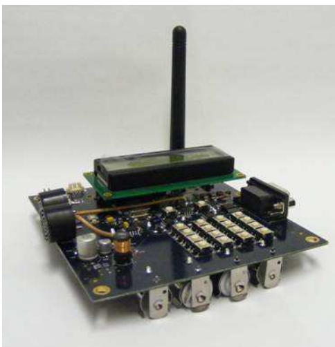
Figure 2. The prototype of an ultrasonic beacon for positioning sensors or mobile sensors underground, together with its housing. The beacon would normally be deployed on the hangingwall.
