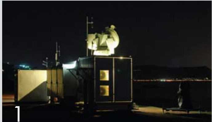
1: The MECORT mobile radar laboratory deployed in False Bay in the Western Cape for maritime target and clutter measurements.
