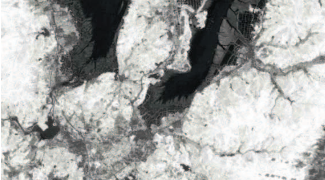
◆ FIGURE 26. Part of the NDVI scene generated for Huangdun Bay to improve the land classification. This highlights the forest/crop regions, whereas urban and bare regions are darker.
