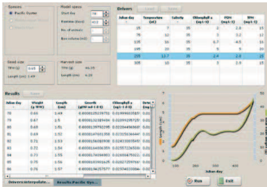
◆ FIGURE 96. WinShell, a simple web-based screening model for individual shellfish growth
