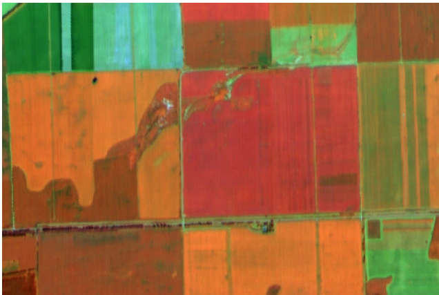
Figure: Original hyperspectral image. Reflectance values for bands 29 ( 0.988 \mu\text{m} ), 39 ( 1.727 \mu\text{m} ) and 1 ( 0.496 \mu\text{m} ).
