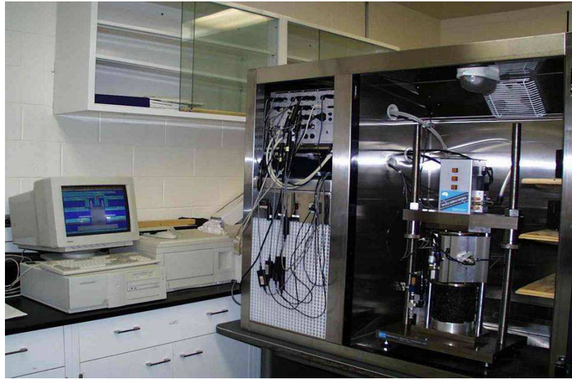
FIGURE 2.3 RaTT Cell Setup in the Temperature Controlled Environmental Chamber.
