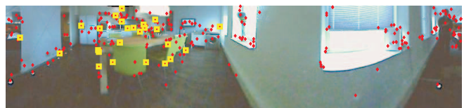
Fig. 1. Typical panoramic image showing all the SIFT features in red with the persistent SIFT features highlighted in yellow.
