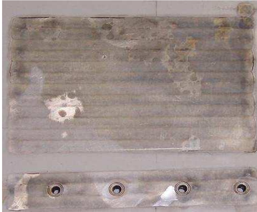
Figure 5: Honeycomb Aluminium plate after irradiation scan
