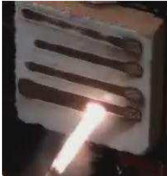
Figure 3: Decoating of a 180 to 230 \mu m thick multi-layer painted surface
