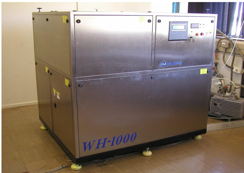
Figure 2: WH1000 High power transversely excited atmospheric (TEA) CO 2 laser
