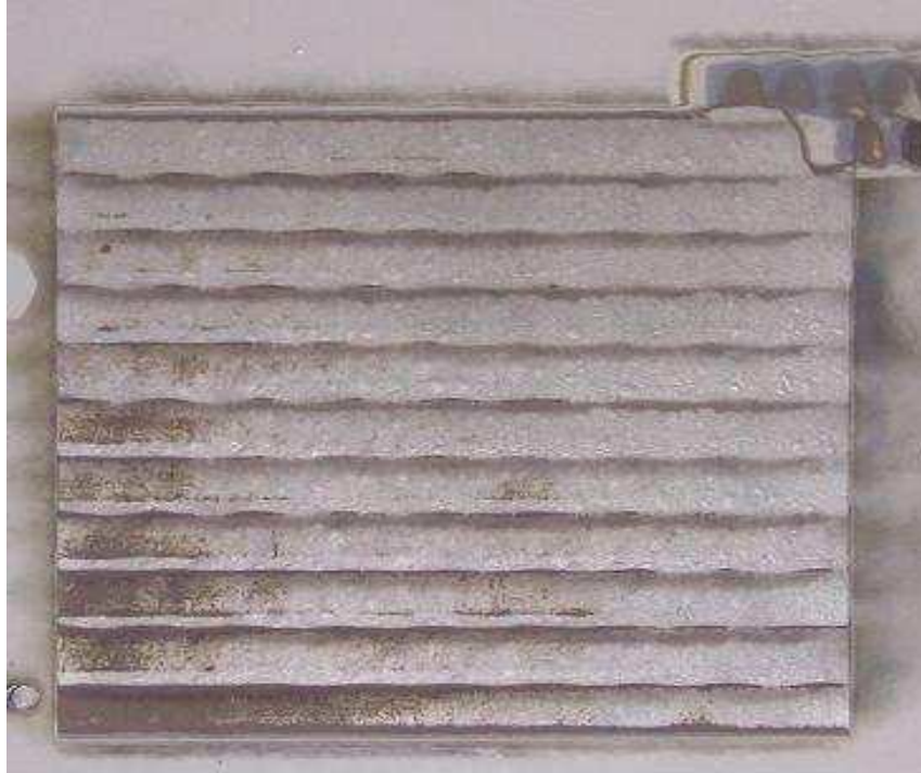
Figure 6: Paint stripping of honeycomb composite aircraft panels
