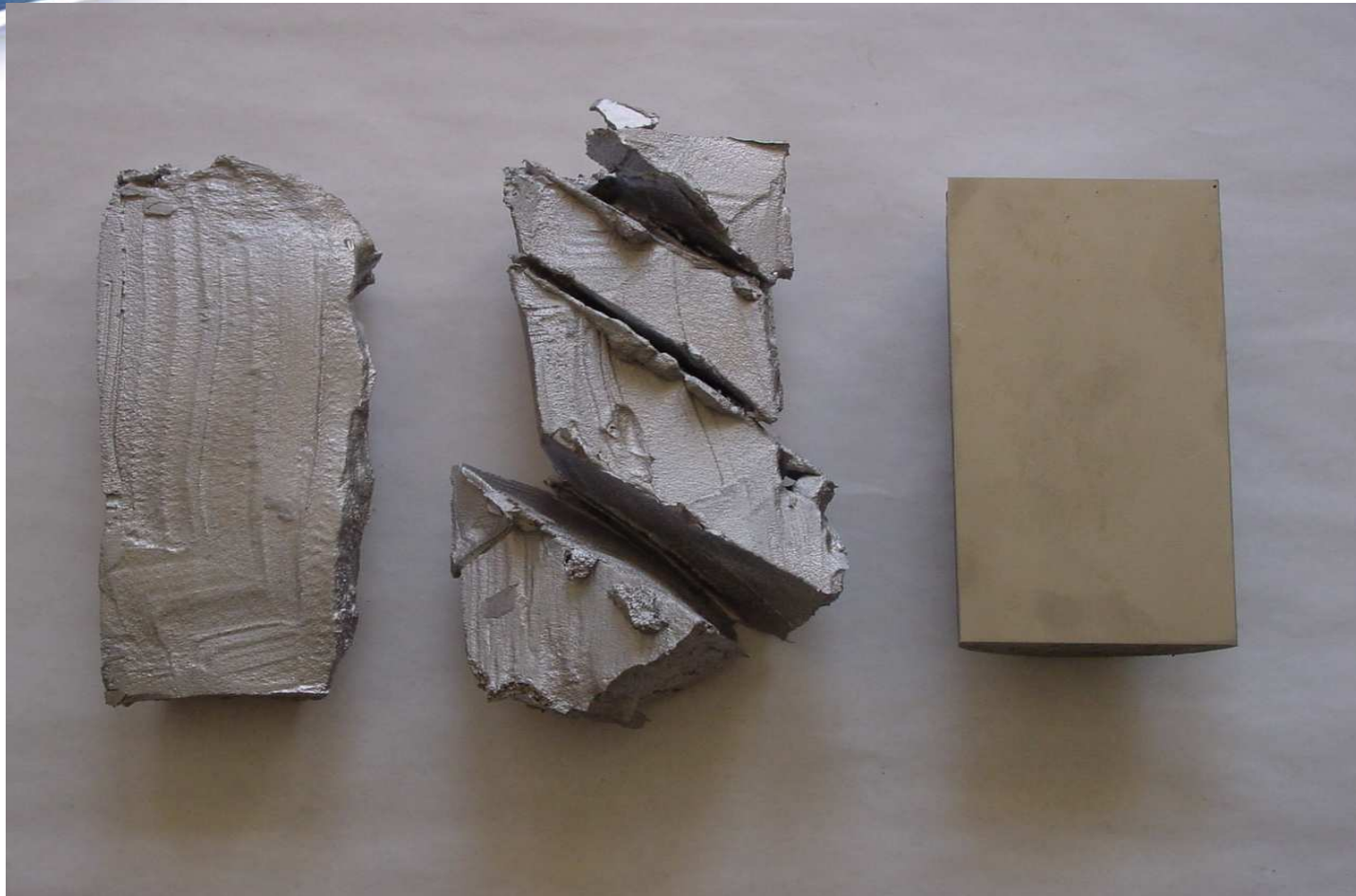
Longitudinal section and two kitchen knife tests of the 90 mm billets
