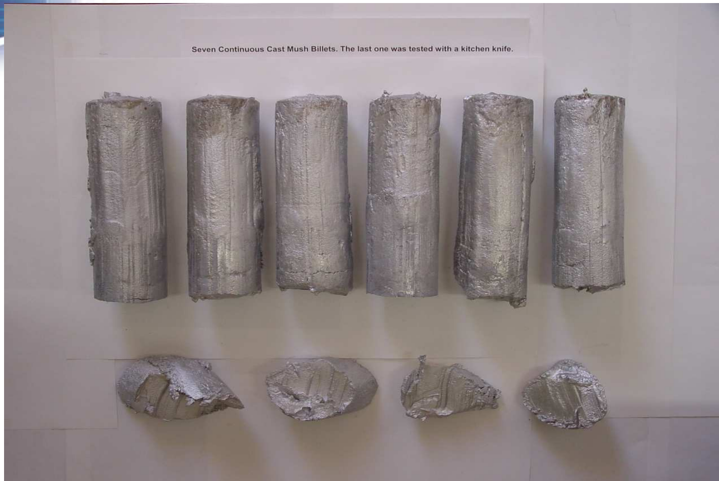
Seven continuous cast billets 60 mm diameter and 180 mm length, casting No p1. The last one has been “kitchen knife tested”
