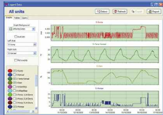
The 'SmartHistory' software module, showing collected manufacturing data
