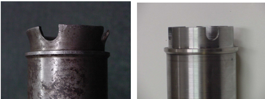
Figure 3: Damaged and repaired distance sleeve
