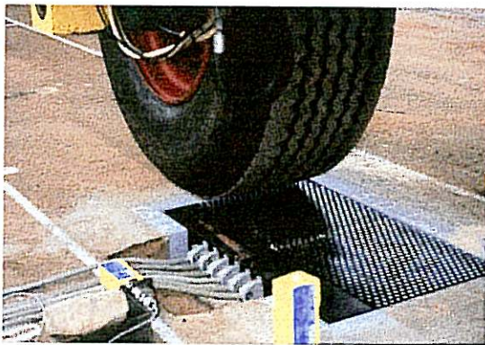
Plate 1 : Images of the Vehicle-Road Surface Pressure Transducer Array (VRSPTA) as used under the Heavy Vehicle Simulator (HVS). The tyre tested here is a wide base 425/65 R 22.5 type.
