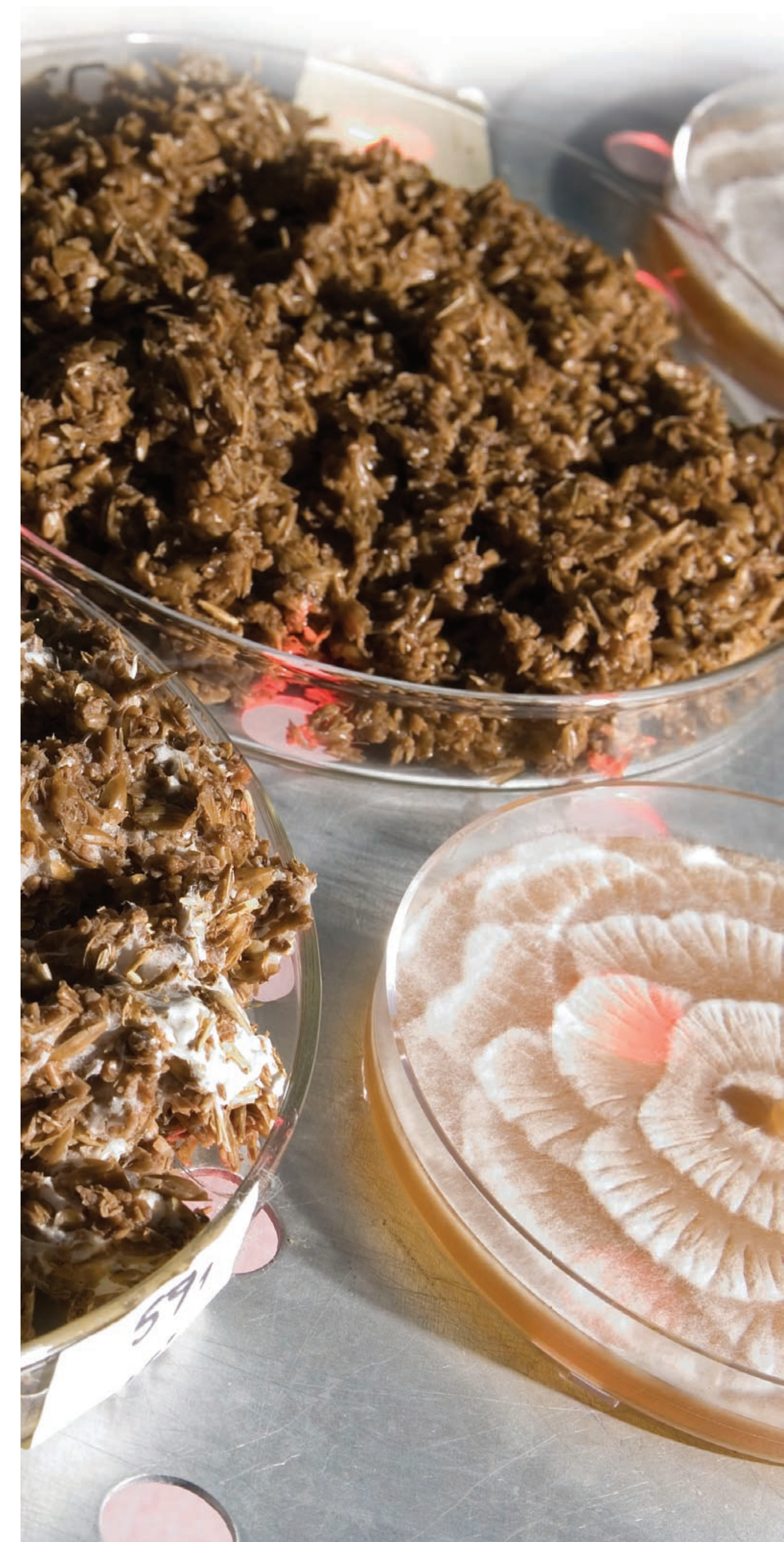
Figure 4: The production of EPA on sunflower press cake by fermentation with Mortierella fungi
